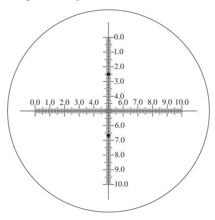
The position of the oil drop at the start and end of a 120s time interval is indicated by the black dots.
