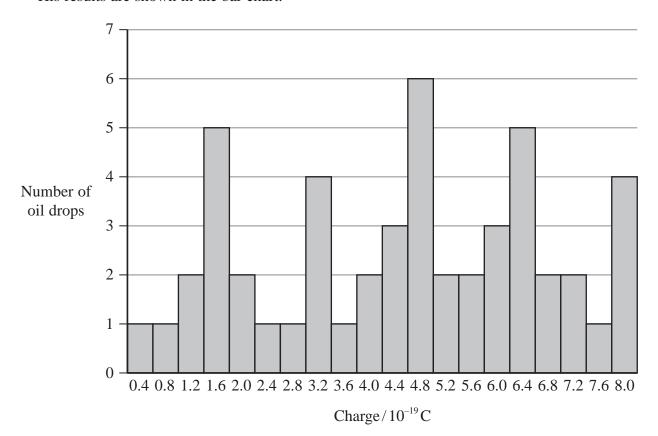
The student predicted that the charge on each oil drop would be a whole number multiple of the charge on an electron.
