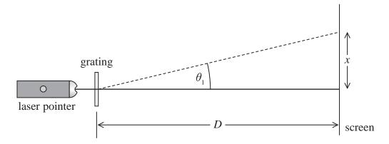
A diffraction pattern was produced on the screen. The distance between the first order maximum and the central maximum of the diffraction pattern was x. The distance between the diffraction grating and the screen was D.
