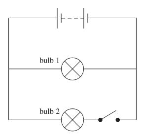
Each bulb has a normal working power of 40 W when a potential difference (p.d.) of 12 V is applied.
